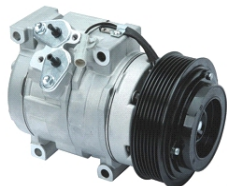
HIACH(OPPOSITE DIRECTION) OEM#: TYPE: 10S15C PULLEY: 7PK 120mm VOLTAGE: 12V
